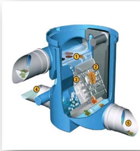
Figure 14.3 Mechanical roof wash device. (Courtesy: Graf Corporation).
